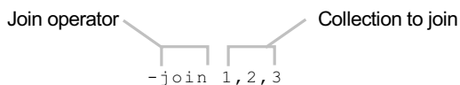
Figure 4.10 The unary join operator allows you to join a collection of objects into a single string with nothing between each element.
