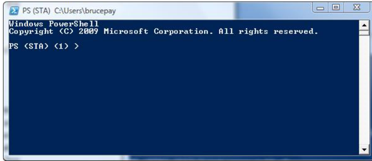
Figure 1.3 When you start an interactive PowerShell session, the first thing you see is the PowerShell logo and then the prompt. As soon as you see the prompt, you can begin entering commands.
